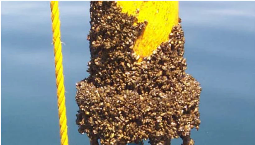
Zebra mussels fouling a marine sensor (Image: NOAA/Wikipedia)
